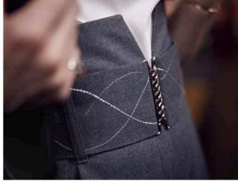
This simple, elegant belt features a chainstitch embellishment, sewn using the PFAFF® admire™ air 7000 coverlock machine. The chainstitch is a 2-thread stitch, created using the machine's chainstitch needle and chainstitch looper. By using a heavier weight, decorative thread in the chainstitch looper, the result is a bolder, more pronounced appearance to the stitch.
